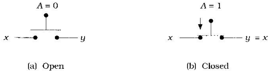
Figure 2.1 Behavior of an assert-high switch
