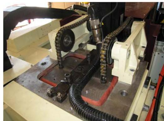
8. Home Machine: Turn function knob to home (See page 4). X, Y, Z Home indicator start to flash. First put rapid rate to F0. Push +Z button. The home light will stop flashing when Z on home position. Push -X, +Y, until all X, Y, Z home light stop flashing. \* (see page 4)
