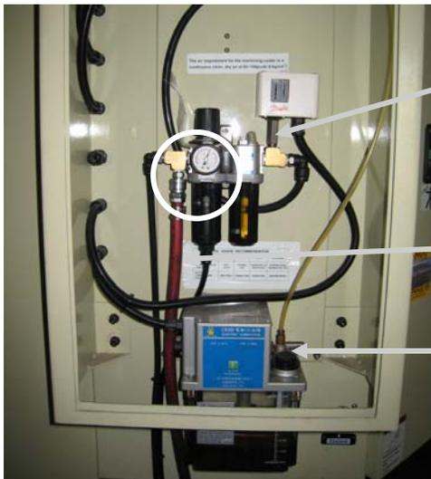
Pull knob up and turn to adjust setting. 90 psi minimum
