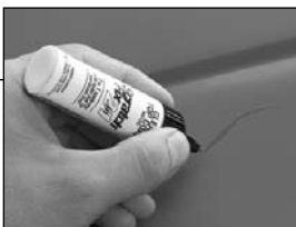
STEP 4: Apply Clear Top Coat
